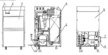
1. Switch 5. Ice Shovel Outlet 9. Water 2. Operation Board 6. Back Panel Tube 3. Door 7. Power Cable 10. Foot Screw Temperature 8. Screw for 11. Water Inlet Tube Sensor Drainage
