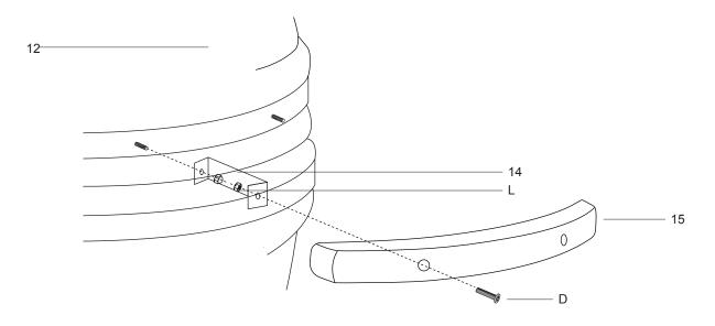
STEP 10 - To attach the handle (15) to the lid of the Kamado Grill (12) start by attaching 2x handle brackets (14) using the 2x pre-attached bolts and dome headed nuts. Attach the handle (15) to the brackets (14) using 2x bolts (D) and nuts (L).
