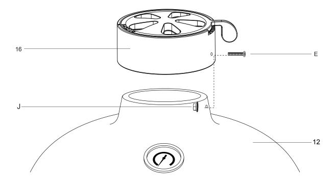
STEP 11 - To attach the top vent (16) to the Kamado Grill (12) place it on top and align both the bolt holes. Secure using 1x bolts (E) and nuts (J). Ensure that the top vent bolt is on the left hand side when assembling it.
