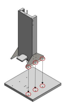
Place and screw the top of the unit to the sheet metal shown in the picture, corresponding to the connection points on the unit.
